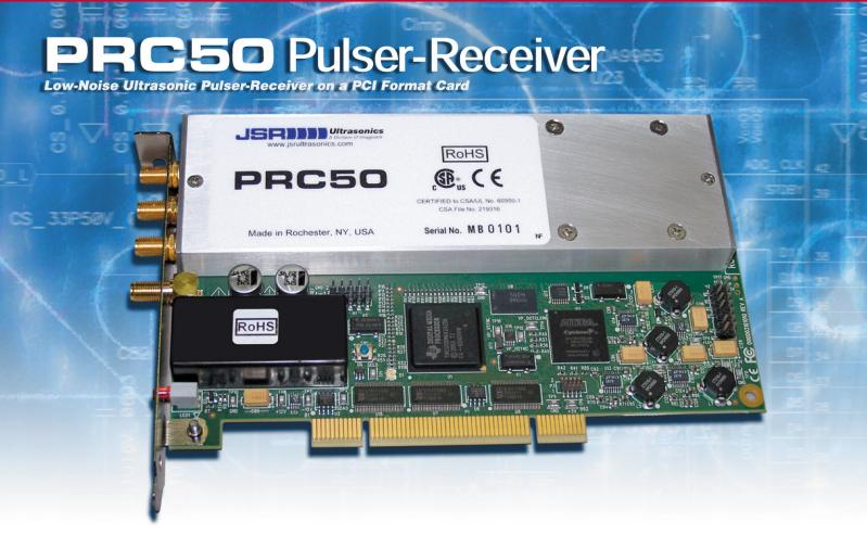
he PRC50 is a versatile single-channel Pulser-Receiver on a half-length PCI card. It is ideal for use in PC-based ultrasonic testing and inspection systems, and its small size and low power consumption enable systems to be implemented using portable computers. The PRC50 is provided with turnkey control software for Windows. A Software Development Kit and Programmer's Manual are provided for the development of custom applications.
